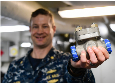
3D printed metal part aboard a US Navy Carrier - Photo courtesy of the U.S. Navy. www.navy.mil
